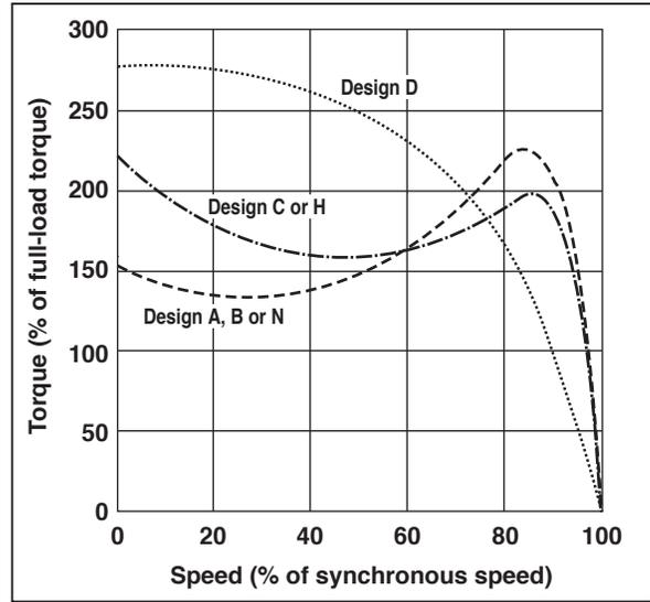
Figure 3. Typical speed torque curves.
